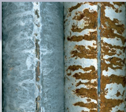
Magnelis® ZM120 welded, not re-protected
